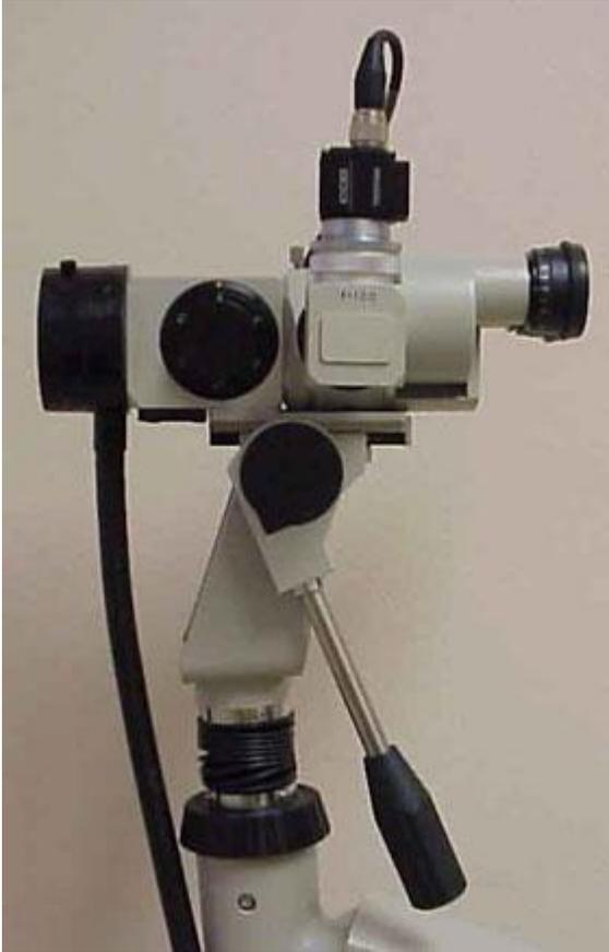
Lower magnification yields a wider view and a greater depth of field for observation. Higher magnification can reveal small features such as abnormal blood vessel patterns and other finer details. As the magnification level increases, the field of view and illumination levels usually decrease. 2
