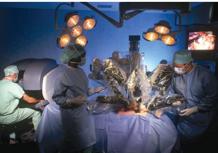
Left, da Vinci Surgeon Console; Center, da Vinci Patient-Side Cart; Right, High-Definition Monitor
